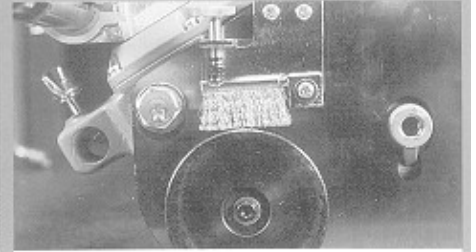
Wheel brush (shown in photograph): S/N60036957 Weight and Support Bar Long type 135mm (5.25") : S/N60031855
